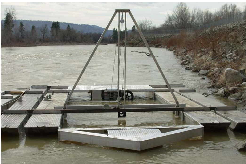
Figure 2. Photo of the 8-foot trap barge illustrating improvements made for the 2007 season. Note the retrofitted debris deflector and supplemental outriggers for extra floatation.
