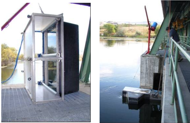
Figure 3. Photographs of Zosel Dam west bank video chute array prior to (left) and during deployment.
